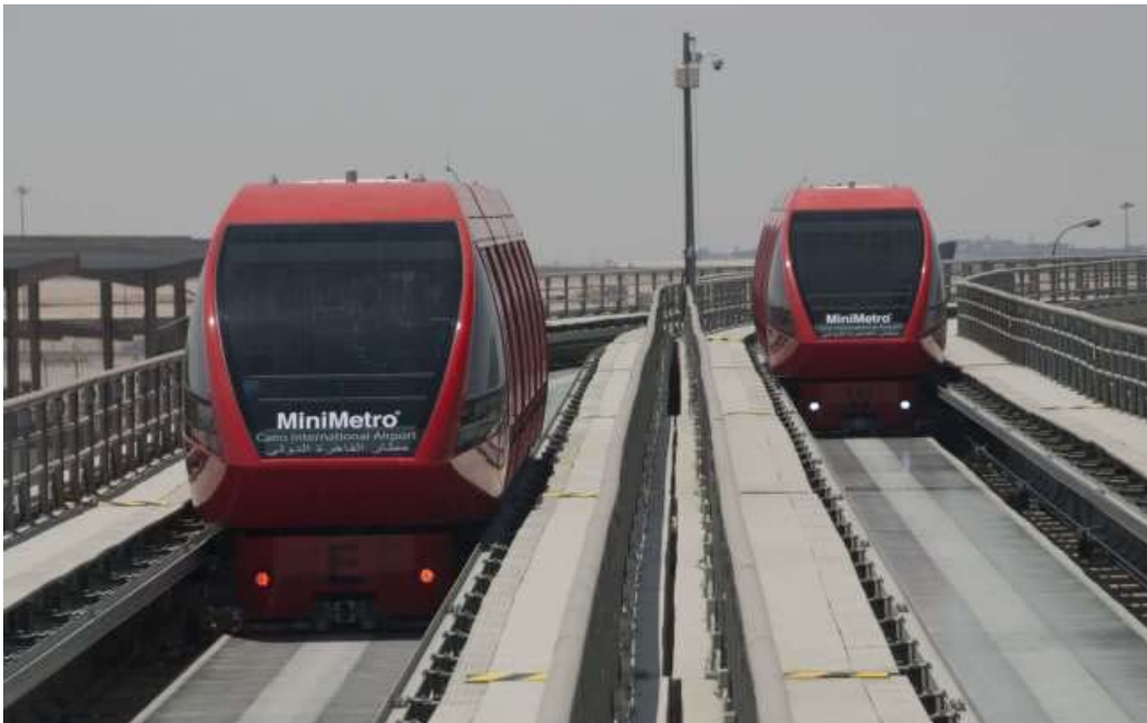
Figure 3.3.2-2 Leitner-Poma MiniMetro utilizing Hovair® air levitation suspension, Cairo Airport, Egypt (Image: Leitner-Poma)
