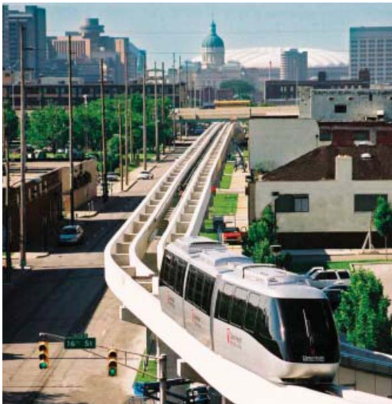
Figure 3.1.5-2 Schwager Davis UniTrak vehicle at IU Health, USA (Image: SDI)
