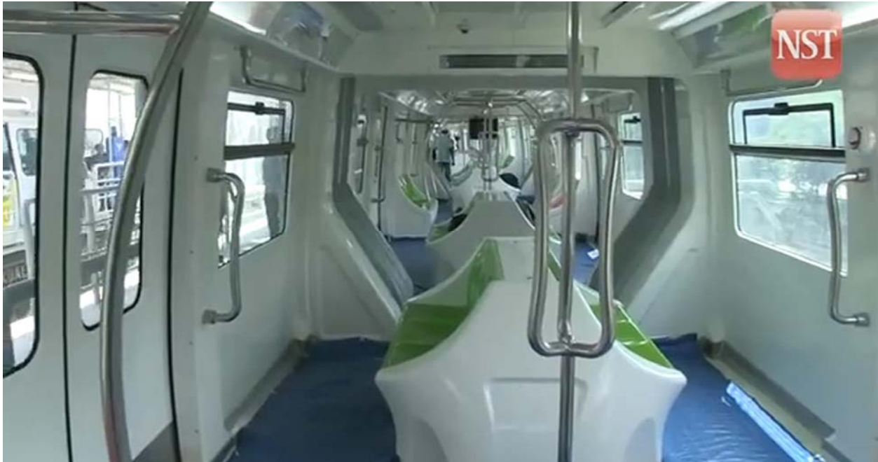
Figure 3.2.3-3 Scomi SUTRA Monorail vehicle interior, Manually-operated with driver (Image: Scomi/NST)
