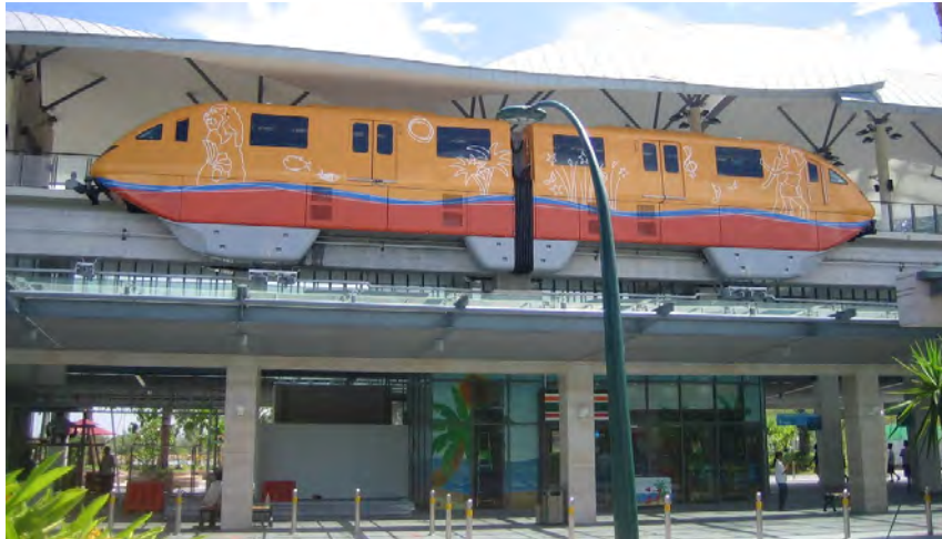
Figure 9. Hitachi Sentosa Express Monorail, Sentosa, Singapore (Manually-operated with driver)
