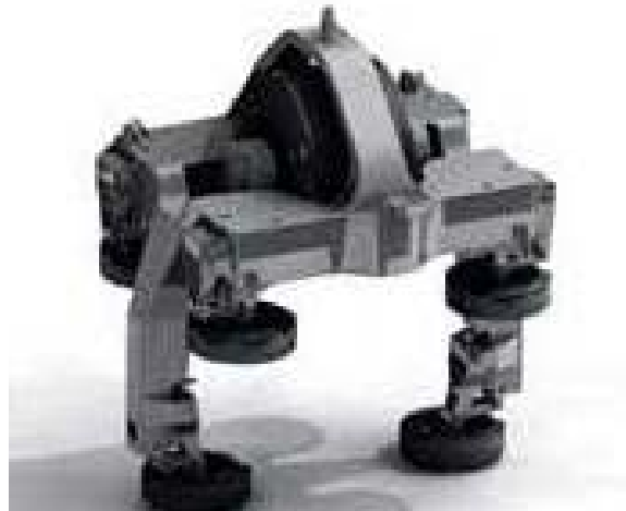
Figure 3.2.3-4 Scomi SUTRA Monorail guidance system (Image: Scomi)
