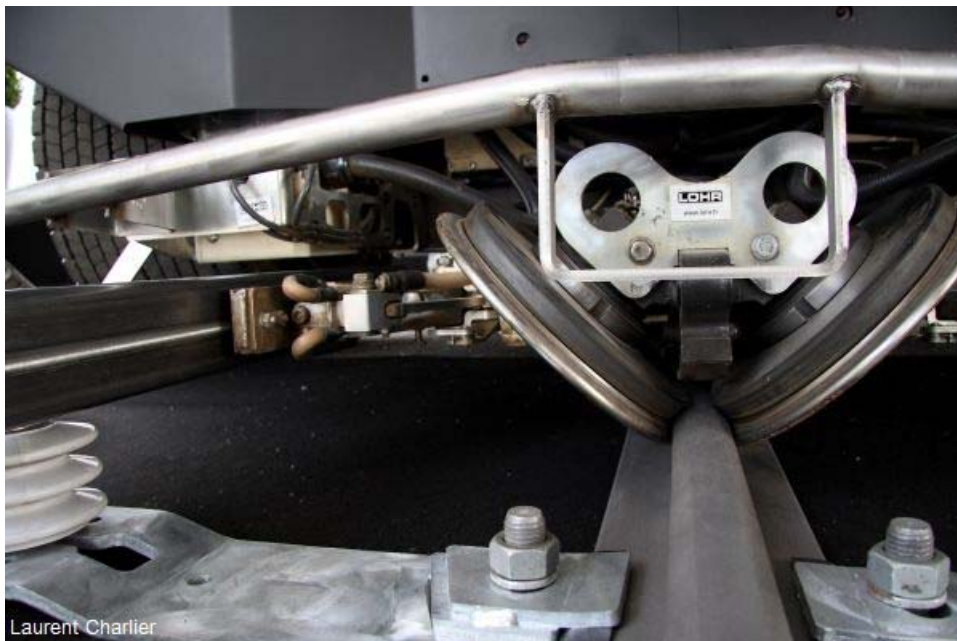
Figure 3.1.6-4 Siemens Airval guidance system on exhibit (Image: Laurent Charlier)
