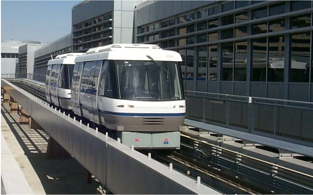
Figure 3.3.2-1 Leitner-Poma (formerly Poma Otis) MiniMetro utilizing steel wheels/steel rail guidance, Minneapolis-St. Paul Airport, MN USA (Image: Lea+Elliott)
