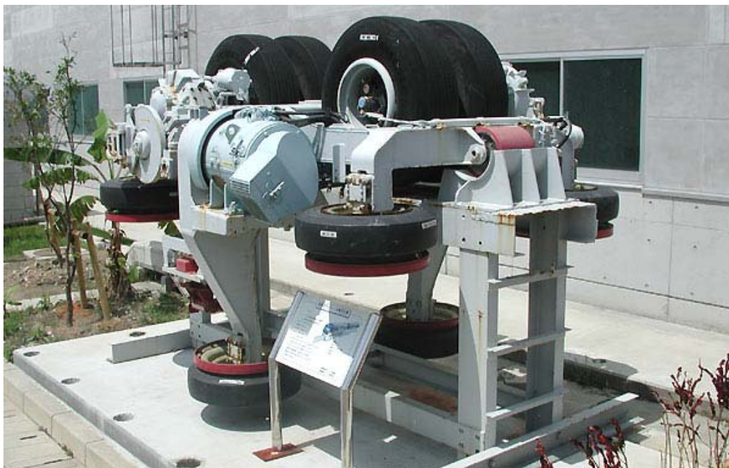
Figure 3.2.2.1-4 Hitachi Standard Monorail guidance system (Image: Hitachi / The Monorail Society)
