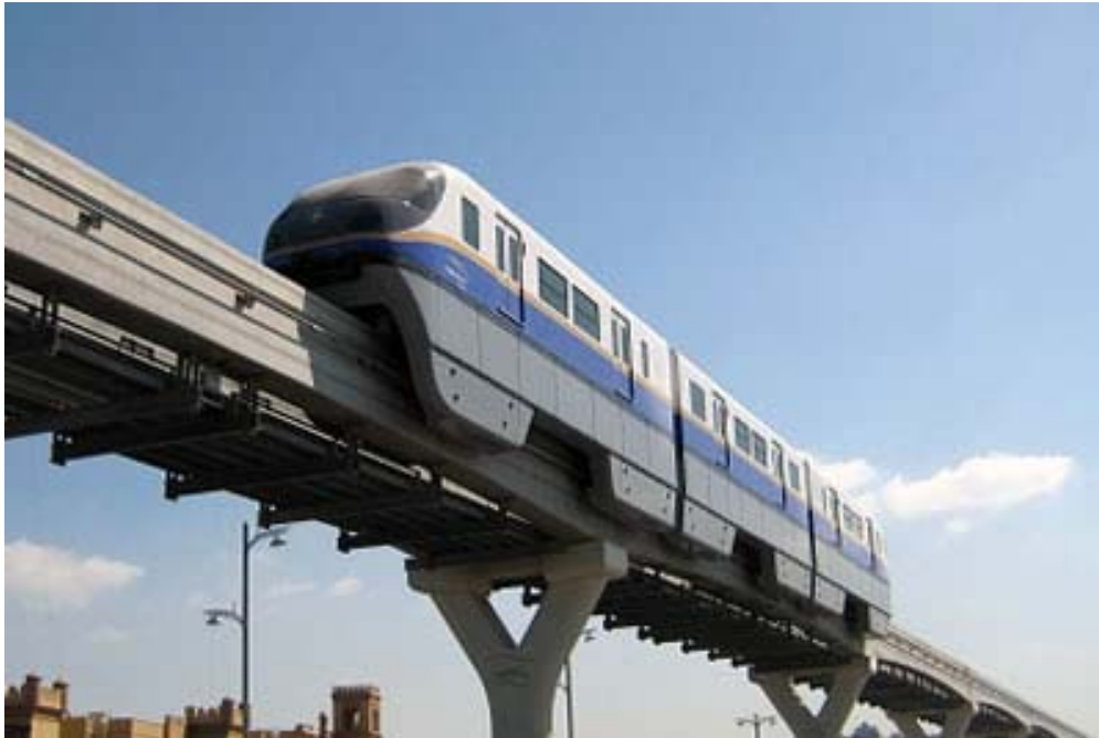
Figure 3.2.2.1-1 Hitachi Palm Jumeirah Monorail, Dubai, UAE, Fully-automated without driver (Image: Hitachi)
