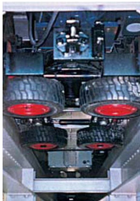
Figure 3.1.5-4 Schwager Davis UniTrak guidance system (Image: SDI)
