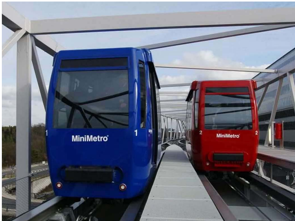
Figure 3.3.2-5 Leitner-Poma MiniMetro small vehicle on The Sqaire metro, Frankfurt Airport, Germany (Image: Leitner-Poma)
