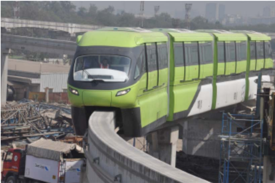
Figure 3.2.3-1 Scmi SUTRA Mumbai Monorail, India, Manually-operated with driver (Image: Scmi)
