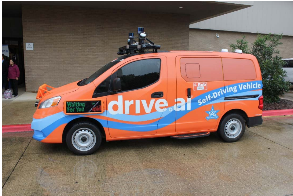
Figure 3.8.2-1 Drive.ai Nissan NV200 van with sensors, Arlington, Texas (Image: Lea+Elliott, Inc.)
