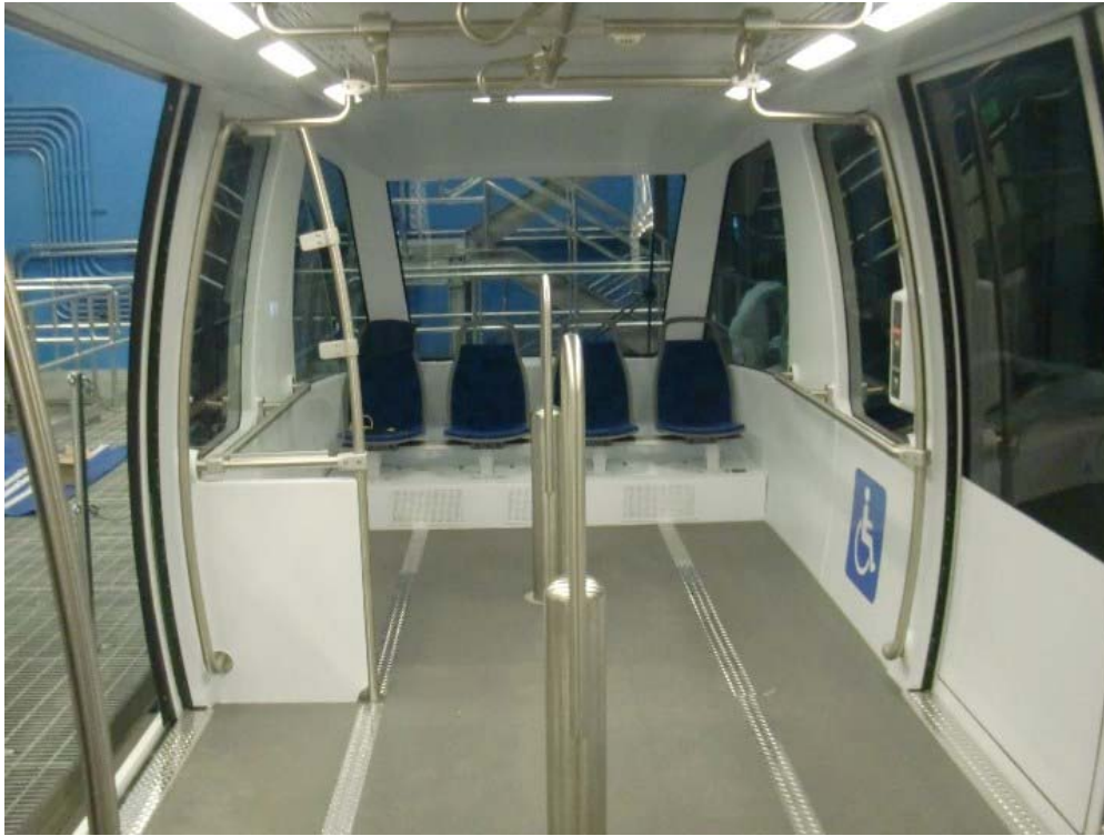
Figure 3.3.1-3 Doppelmayr Cable Liner Shuttle vehicle interior, BART TO OAK, Oakland, CA USA (Image: Lea+Elliot)
