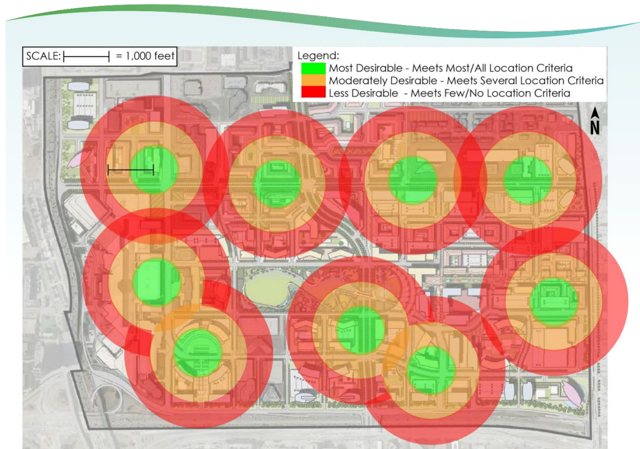
Figure 6-1. Parking Structure Site Selection Analysis
